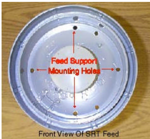
Figure 4. SRT feed horn
